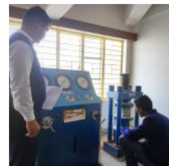
Compressive Strength Machine
