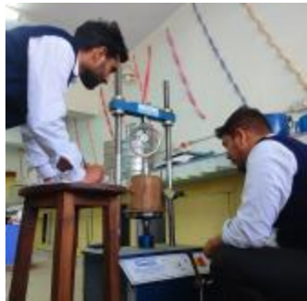
California Bearing Ratio Test
